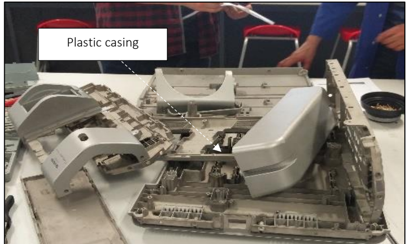
Figure 7: Injection Moulded plastic casing
