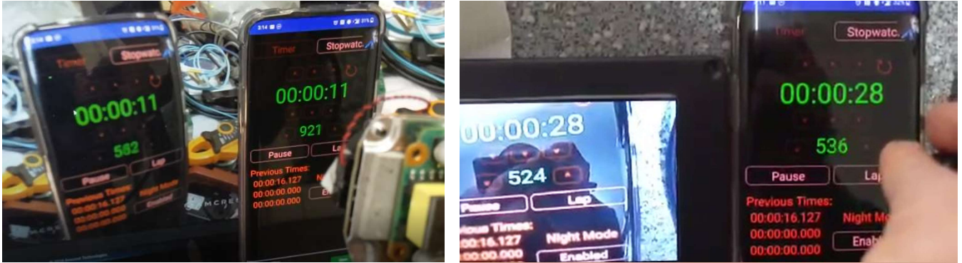
Figure 17: results of the camera latency tests with the PoE camera left and analogue right. Cameras are to the right of the images watching the phone. The phone is on the right and the camera feed is the phone on the left.
