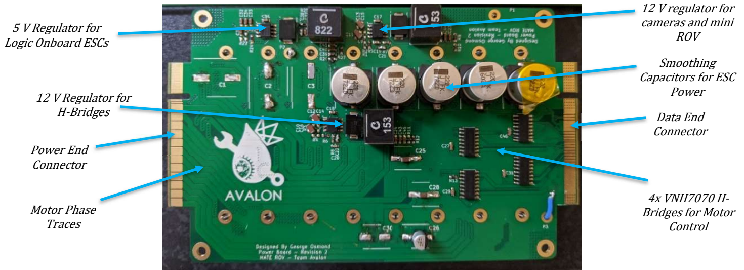
Figure 20: Fully Populated Power Board - Top
