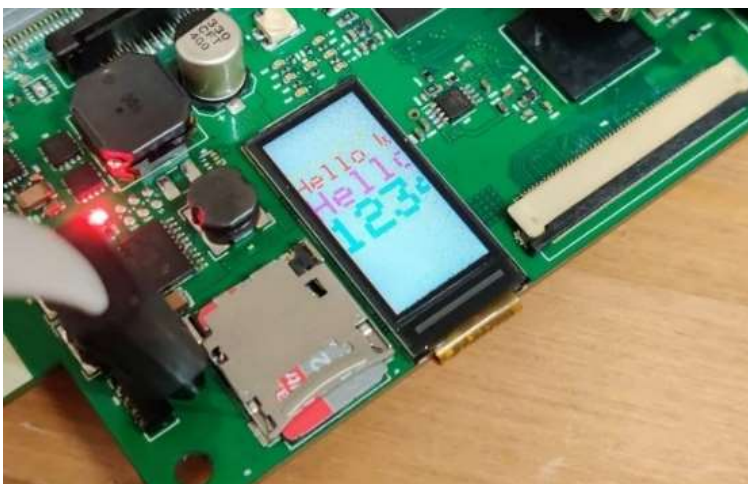
Figure 12: debug screen in operation with a test card
