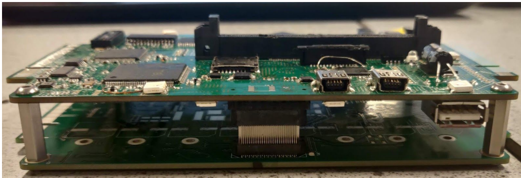
George 2: Showing the board-to-board connector between the data and power board
