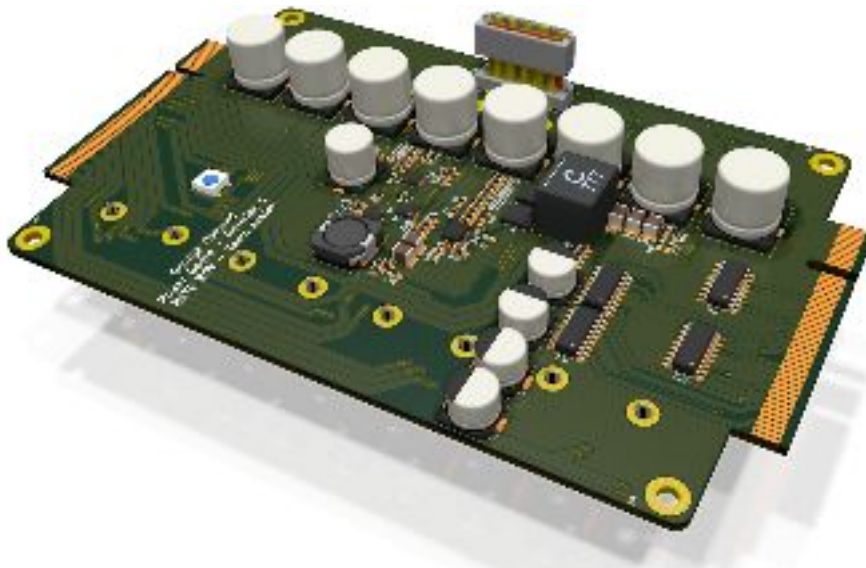
Figure George 1: Render of Revision 1 Power PCB
